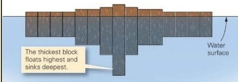
(c) Because of isostasy, blocks of wood floating in water sink to a depth such that the mass of the water displaced is the same as the mass of the block.
